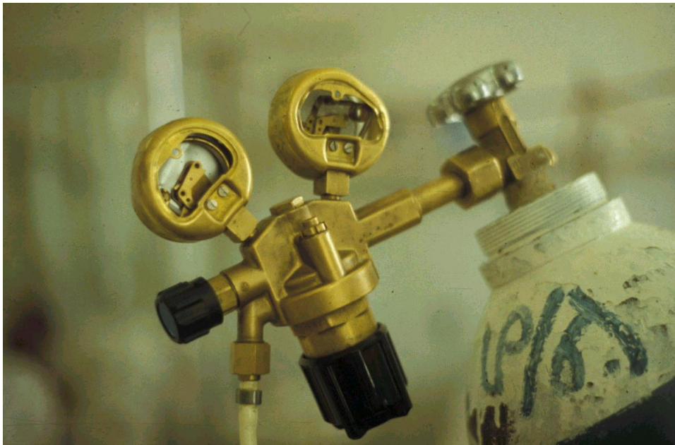
Picture 2. Defect oxygen pressure regulator (before 1997).
